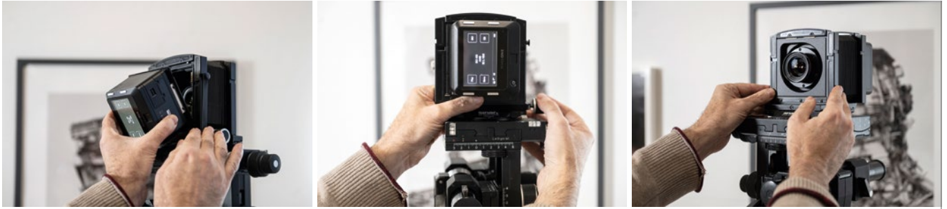
Optionally, aperture bodies or X-Shutter lenses can be combined with the Phase-One-IQ4-Back (Pictures: © Natalia Kepesz).
